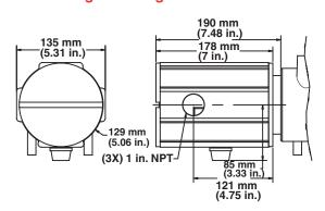
**NEMA 1 Housing With Double Pole Thermostat**
