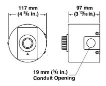
**NEMA 4 Housing With Single/Double Pole Thermostat**
